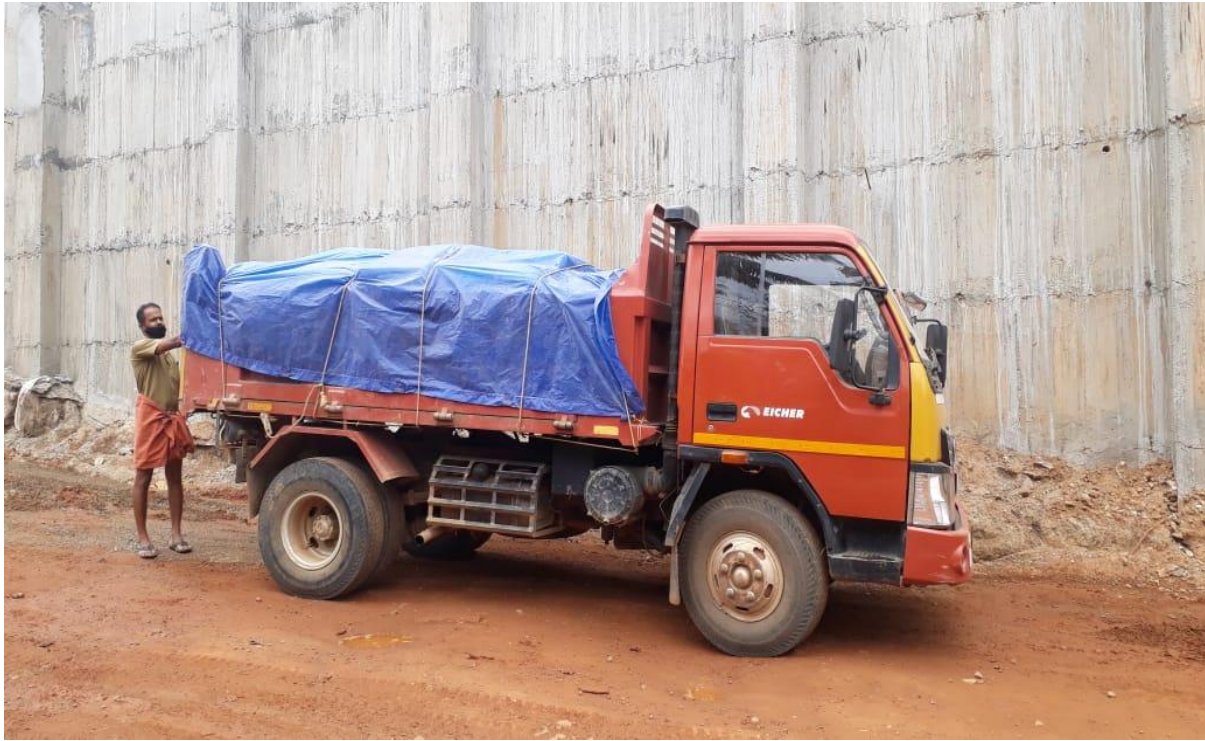
Plate G-20: Transportation materials in covered truck
